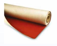
The silicone rubber coating is completely impervious to water, moisture, hydraulic oils. When exposed to high temperatures or molten splash for extended periods, the coating transforms into a silica refractory crust.
