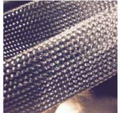
EP22 FR is flame retardant and will operate at temperatures within the range -50°C to +150°C. It also has excellent resistance to damage by mechanical abrasion and repeated flexing. The monofilaments will resist attack by salt water, oils and
